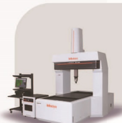
LEGEX-9106 Ultra-high Accuracy CNC Coordinate Measuring Machine Accuracy: E_{\text{a}}, MPE=(0.28 + L/1000) \mu\text{m}
